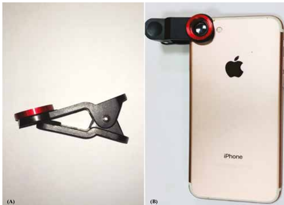
Figure 1: (A) Macro lens with a customized clip. (B) Macro lens with the clip attached on the smartphone.
